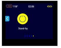
On the fifth page of the main menu it is possible to put the machine in stand by without using the main switch.
