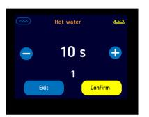
This page allows you to set the water dosing for tea (in seconds) through the "+" and "-" keys.
