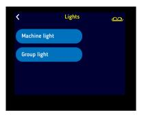
Pressing the "Light" key, will display the following page. It allows switching ON /OFF the machine light indicators.
