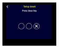
It is possible to program the doses to be used with the enabled keys. If the key is set as "Continuous", programming is not possible. The key appears with an "X".
