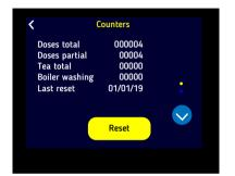
Pressing the "Counters" key, will display the following page. It displays total and partial counters present on the machine.
