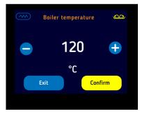
This page allows you to set the boiler temperature (hot water and steam) through the "+" and "-" keys. Save these values by pressing the "Confirm" key.
