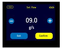
Using the "+" and "-" keys, the dose flow can be set and stored by pressing the "CONFIRM" key.
