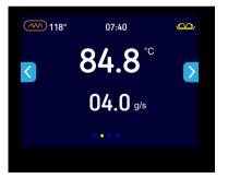
Nn the second page of the main menu, the temperature (in  $^{\circ}$ C) and the coffee flow (in g/s) set in the brew mode are displayed.
