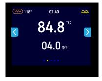
The second page of the main menu displays the set temperature (in  $^{\circ}$ C) and the coffee flow (in g/s) set when dispensing with key.
