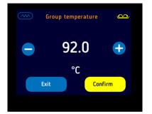
The keys "+" and "-" allow you to set the temperature of the unit and to save it by pressing "CONFIRM".
